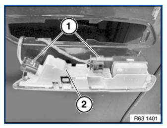
Unlock plug connections (1) and disconnect.
