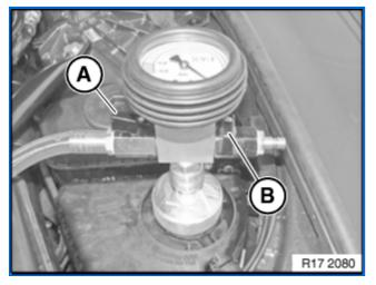
Position the filling unit container at the same height as the coolant expansion tank.
