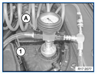
Then open shutoff valve (A) until the filling hose (1) is free of bubbles. Close shutoff valve (A) again. The filling hose (1) is vented in this way.
