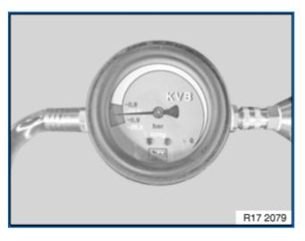
The cooling system must hold the vacuum for 30 seconds. If the needle in the vacuum meter falls, this indicates a leak in the cooling system.
