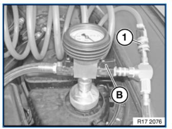
Connect compressed air (1) and open shutoff valve (B).
