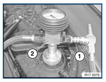
Connect venturi nozzle (1) to filling unit (2).
