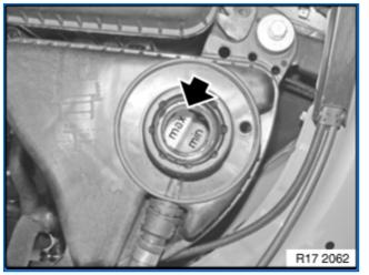
Adjust coolant level to maximum.
