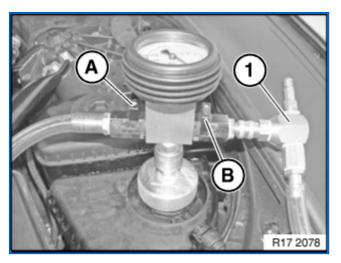
Both shutoff valves (A) and (B) must be closed. Then seal Venturi nozzle (1).
