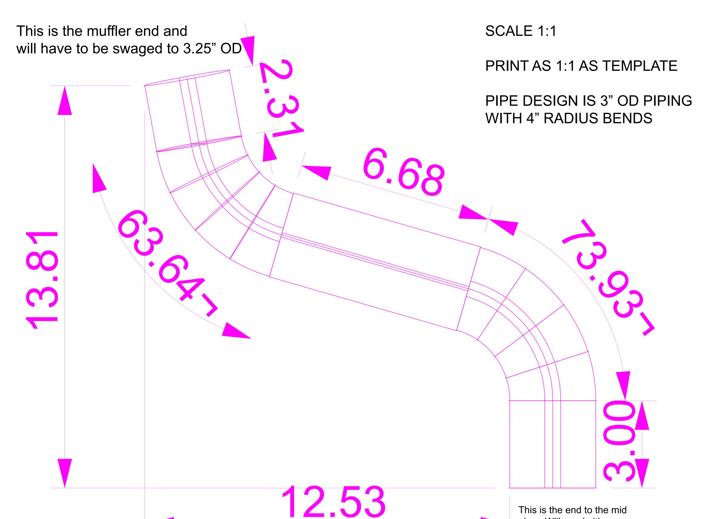
This is the end to the mid pipe. Will need either a 3" OD to 2.75" OD reducer welded in lieu of 3" section or swage the factory pipe from the engine to fit the 3" pipe. This can be made longer, then cut to length if needed.
