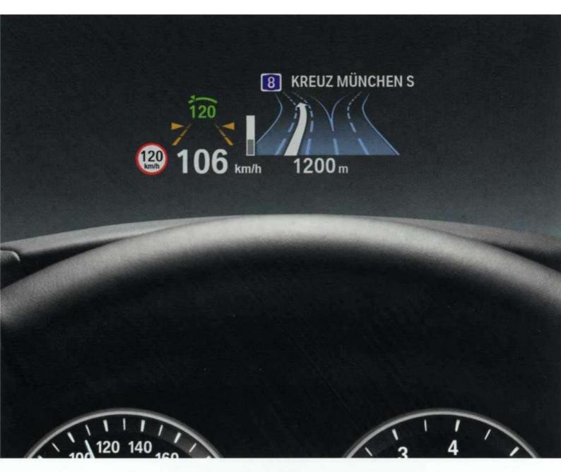
□ 610 Head-up Display in full colour. Projects important information such as the current road speed directly into the driver's field of vision. For the first time, all Head-up Display data are shown in full colour, making information more precise and easier to process. Navigation instructions, Lane departure warning messages, Speed limit display, Check Control, and warnings from the Night Vision pedestrian recognition system can also be displayed.
