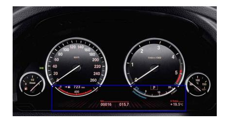
From March 2011 production, full black panel technology is available when Head-up Display (option 610) is selected. The speedometer and rev counter dials also now feature black panel technology as well as a larger 9.2" lower display as highlighted.
