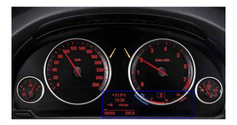
The standard instrument display features partial black panel technology – 5.7" area highlighted above. The speedometer and rev counter dials do not feature black panel technology.
