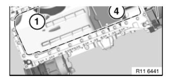
For vehicles with four-wheel drive or automatic transmission, bolts of different lengths are installed for mounting the oil sump.
