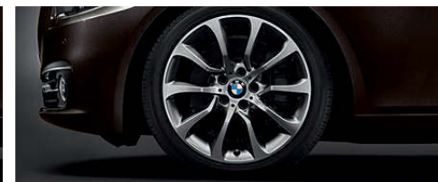
19" light alloy wheels Turbine styling 453 in Bicolor Ferric Grey with mixed, runflat tyres. Front: 8.5 J x 19 with 245/40 R 19 tyres. Rear: 9 J x 19 with 275/35 R 19 tyres.
