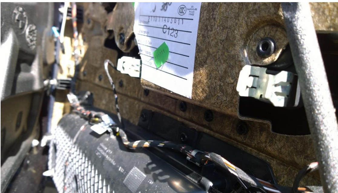
Fig 22 – Those central vice like clips! Remember don't pull outwards!
