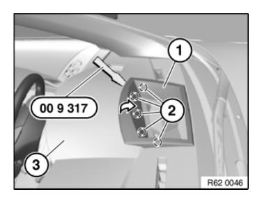
Lever out trim for Head-Up Display (1) with special tool <u>00 9 317</u> at mounting points (2).
